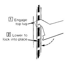
To replace shelves: Select desired shelf height. With shelf front raised slightly, engage top lugs in tracks at rear of cabinet. Then lower front of shelf until it locks into position.
